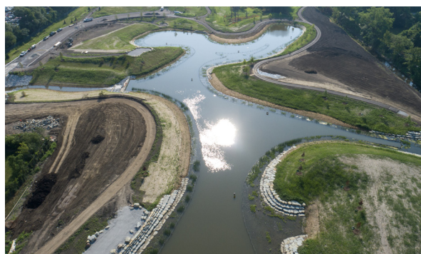
Flood control reservoirs , which temporarily store water from rivers and streams during storms.
