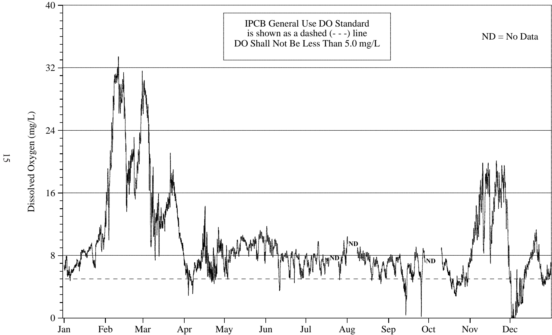
FIGURE 2: DISSOLVED OXYGEN CONCENTRATION MEASURED HOURLY AT MAIN STREET ON THE NORTH SHORE CHANNEL FROM JANUARY 2006 THROUGH DECEMBER 2006
