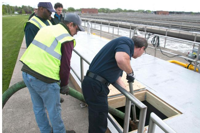
*MWRD Environmental Specialist Jim Schaefer takes a sample of the brewery waste being pumped into a storage tank at the Stickney Water Reclamation Plant in Cicero, IL. The brewery’s high strength organic material will help the MWRD recover more phosphorus during the water treatment process.*
