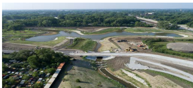
The second phase of the Robbins Heritage Park and Midlothian Creek Restoration project is approaching completion. Located near 137th Street and Kedzie Avenue, it includes a stormwater park, a pond, and conveyance improvements. The project is designed to mitigate flood damage for approximately 100 homes, businesses, and other structures in the surrounding area.
