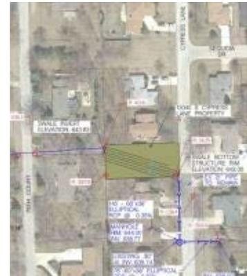
**Project Description** This project will involve the demolition of a property at 13040 South Cypress Lane and the installation of a swale at this location, along with the installation of a new downstream storm sewer and an outfall to Navajo Creek.
