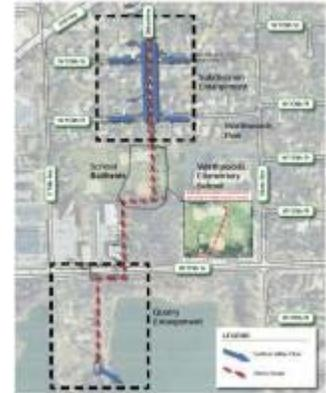
**Project Description** This project will construct a swale and a 24-inches to 72-inches storm sewer, in the vicinity of 112th Place and Beloit Avenue, with an outlet to Lucas-Berg Quarry in the Village of Worth. The project is in the Calumet-Sag Channel Watershed. The Village of Worth will be responsible for ownership and maintenance of the improvements.
