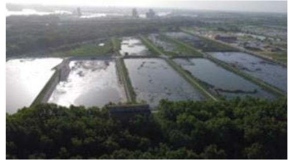
**Project Description** Many of the biosolids lagoons at the Calumet WRP still have the original clay-lined bottoms that over time have been compromised due to the use of heavy equipment to remove and process the biosolids for beneficial reuse. Services are required to restore the lagoons to their original slope. This project will provide restoration that includes regrading and adding material.
