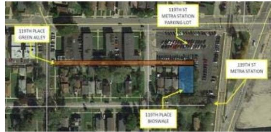
**Project Description** This project is for the City of Blue Island to construct a new bioretention area in a vacant, low-lying lot and a permeable alley using permeable pavers. The City of Blue Island will be responsible for operations and maintenance.
