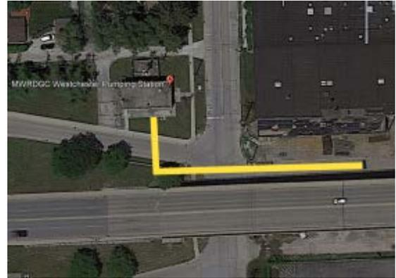
**Project Description** This project entails the installation of a 27-inch diameter sewer in order to provide relief to the Berkley-Hillside Intercepting Sewer and Broadview-Bellwood Intercepting Sewer during wet weather by diverting flow to the Roosevelt Road leg of TARP at DS-D34-AI.
