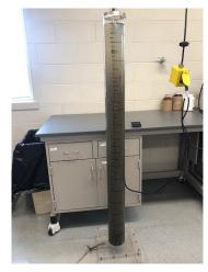
Flocculent Sludge – 5 mins Settling
