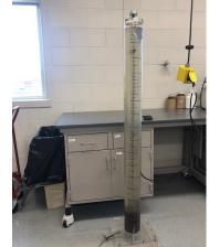
Flocculent Sludge – 30 mins Settling
