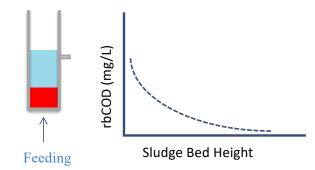
Continuous Flow configuration with high F/M selector
