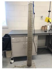
Granular Sludge – 5 mins Settling
