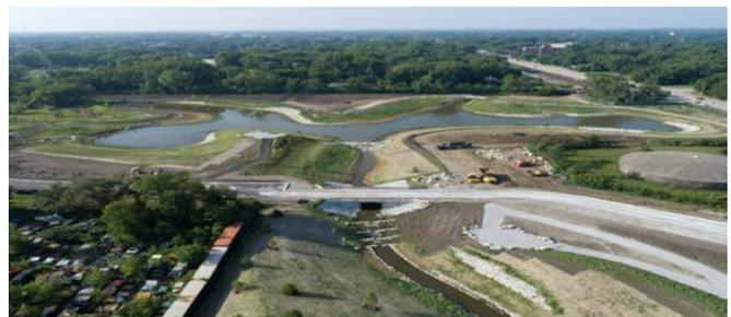
*The second phase of the Robbins Heritage Park and Midlothian Creek Restoration project is approaching completion. Located near 137th Street and Kedzie Avenue, it includes a stormwater park, a pond, and conveyance improvements. The project is designed to mitigate flood damage for approximately 100 homes, businesses, and other structures in the surrounding area.*
