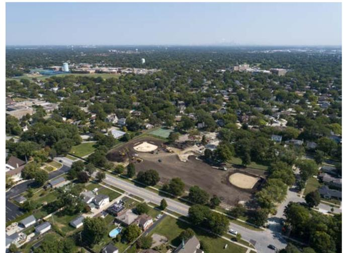
*In Western Springs' Springdale Park, the MWRD is helping fund construction on a supplemental storm sewer system and storage basin that is expected to mitigate flooding in the area through the MWRD's Stormwater Partnership Program. The project benefits approximately 20 homes and two local roads by providing adequate drainage to depressional areas of the neighborhood and detention for excess stormwater runoff.*
