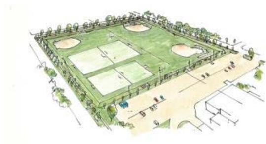
**Project Description** This project will construct stormwater improvements to alleviate flooding in the Village of Oak Lawn. Improvements include the construction of an approximate 27.5 acre-feet stormwater storage facility within the Community High School District 218's ball fields, and upsizing approximately 6,600 linear feet of storm sewers along 105th Street, Kilpatrick Avenue, and Kedvale Avenue. The Village of Oak Lawn will be responsible for long-term operation and maintenance.
