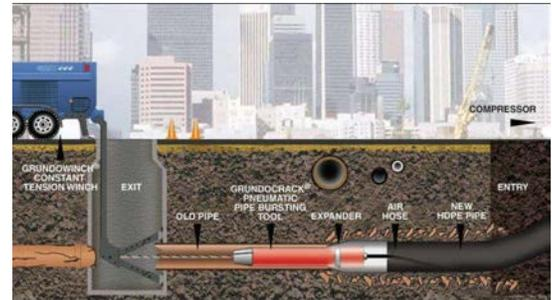
**Project Description** This project consists of the replacement of 1,200 linear feet of 18-inch cast iron pipe and 1,900 linear feet of 20-inch cast iron pipe between the digesters building and the post-digesters building at the Stickney WRP. The sewer replacement will be completed using pipe bursting methods.
