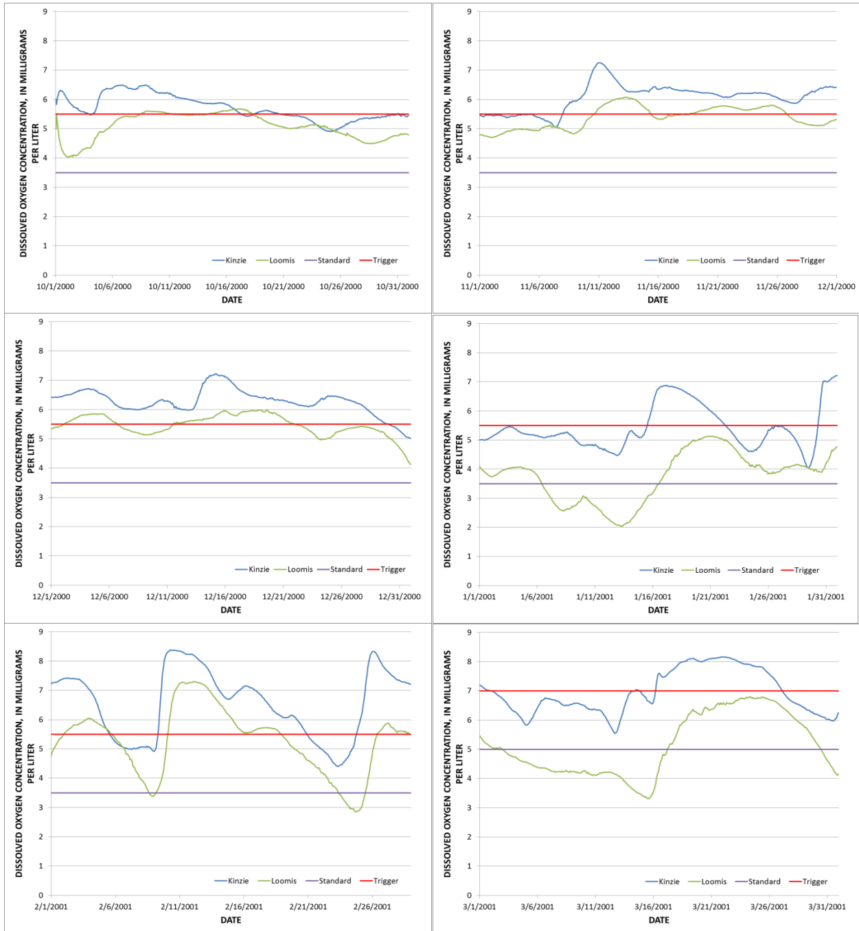
Figure 4.16. Simulated dissolved oxygen (DO) concentration for Water Year 2001 at Loomis Street and Kinzie Street and apparent “trigger” DO concentration at Kinzie Street that results in DO concentrations less than the at any time DO standard at Loomis Street.
