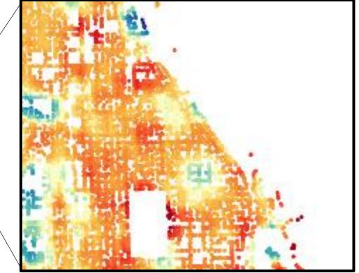
Downscale 1-km climate prediction to submeter street-level air temperature using machine learning.
